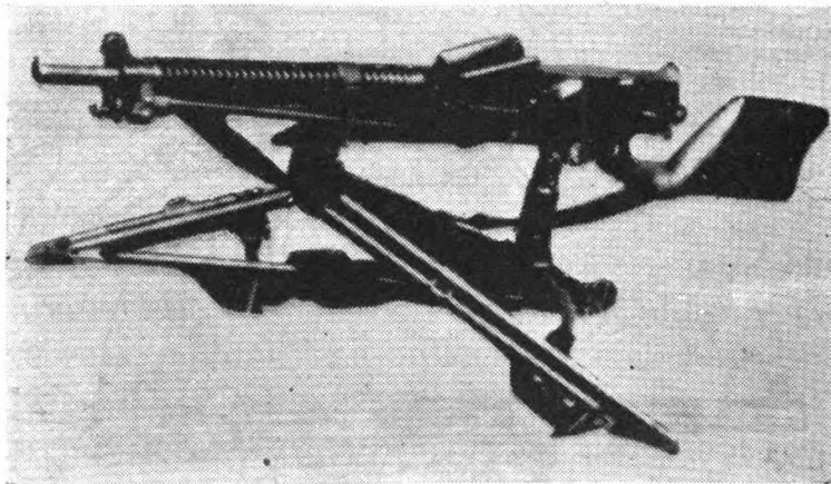
FIGURE 27.—Nambu light machine gun, M1922, with new tripod.
