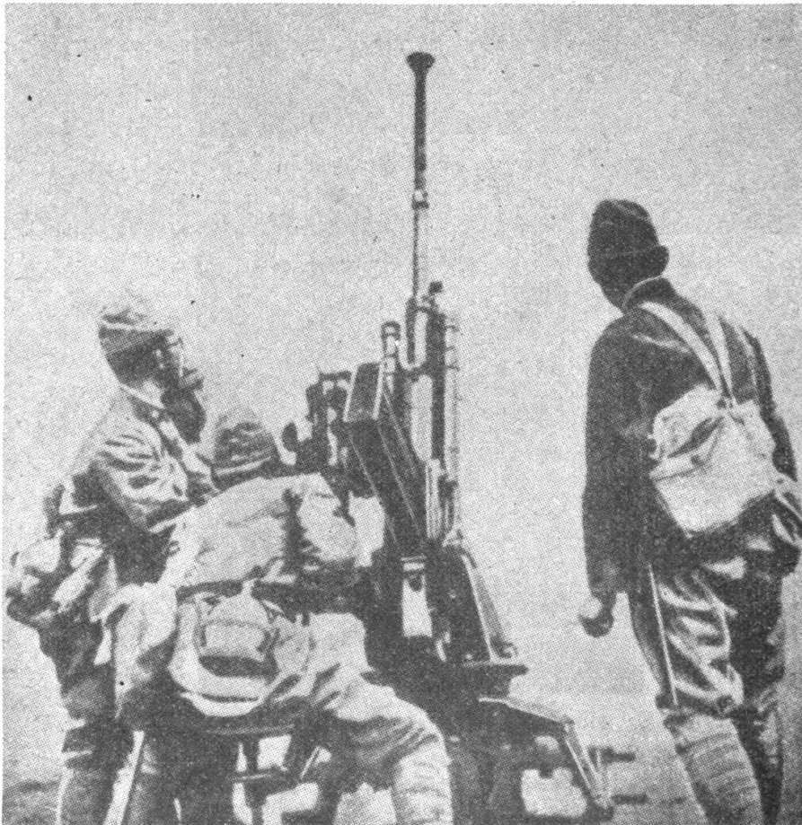
FIGURE 56.—20-mm Oerlikon anti-aircraft and antitank gun.
